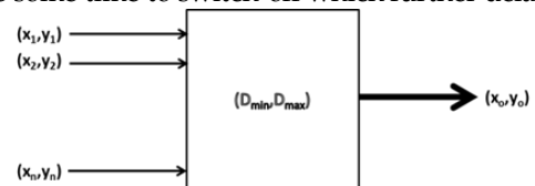
Figure 4: A CMOS logic gate with input and output time slots
